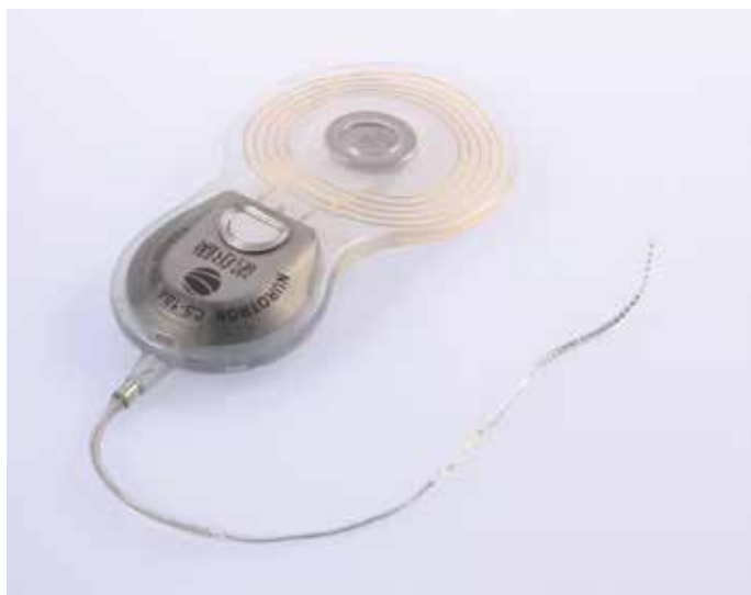
Figure 1. The Nurotron Venus® internal receiver and stimulator (Hangzhou, China). The electrode shown is the standard Nurotron array, 22 mm in length with 24 active stimulus contacts. One reference is a ring electrode located near the titanium case and the other reference is a plate electrode located on the surface of the case.
