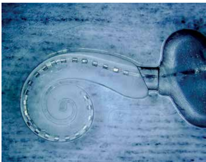
Figure 5. The Nurotron electrode array in a clear cochlear model. To validate the reliability of the electrode carrier, leads, and contacts when subjected to repeated insertions. Test electrodes were mechanically inserted into a clear plastic model of the cochlea. Each electrode was tested 50 times and evaluated for physical damage and electrical performance.
